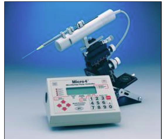
World Precision Instrument's UltraMicroPump II microsyringe pump.
